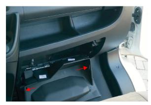
Open the glove compartment and press the clips on the inside to release it so that it can be pulled out completely forwards.
