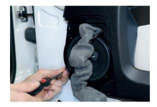
Screw in the JEHNERT upgrade speaker and connect the original plug to the speaker.
