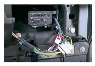
Lay all cables in the space behind the glove compartment.
