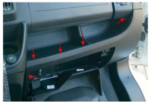
Remove the screw on the inside left under the glove compartment flap, and the screws on the top in the glove compartment cladding.
