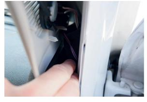
Push the foam sleeve into the area between the dashboard and the A-pillar.
