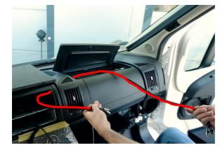
Pull the supplied adapter cable from the radio slot to the storage compartment.
