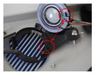
Connect the JEHNERT tweeter, clip it into the holder, and turn it until it locks into place.
