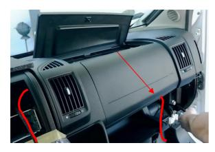
Then run the adapter cable from the storage compartment back underneath into the free space behind the glove compartment.
