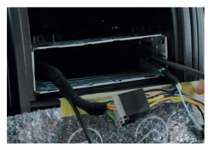
Connect the adapter cable to the radio and Fiat DIN/ISO plug.
