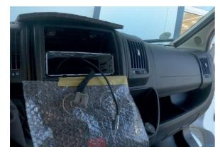
Disconnect all connection cables on the radio and put it to one side.
