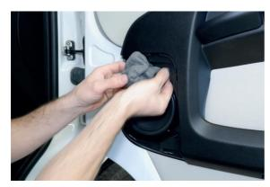
Slide the foam sleeve over the connection and push it through the opening into the space under the cladding.
