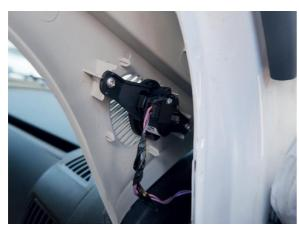
Carefully remove the A-pillar cladding, place it on the dashboard (protect the surface with adhesive tape), and unclip then unplug the existing original tweeter.
