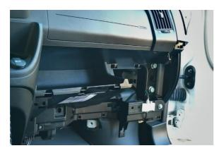
Remove the glove compartment including the cladding part and put it to one side.
