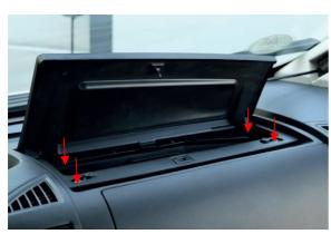
Open the storage compartment, remove the 4 screws inside and put them to one side.
