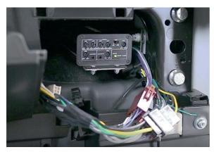
Mount the amplifier on the mounting bracket (AMP V41 CampTec including connection cable) using the original nut with flange as shown and tighten the nut.
