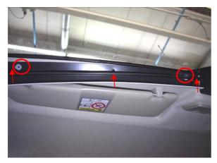
Remove the 2 plastic screws and 3 metal screws at the top in the frame of the REMIS blind.
