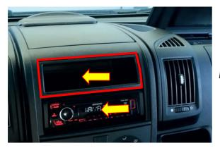
Reassemble the radio and storage compartment.
