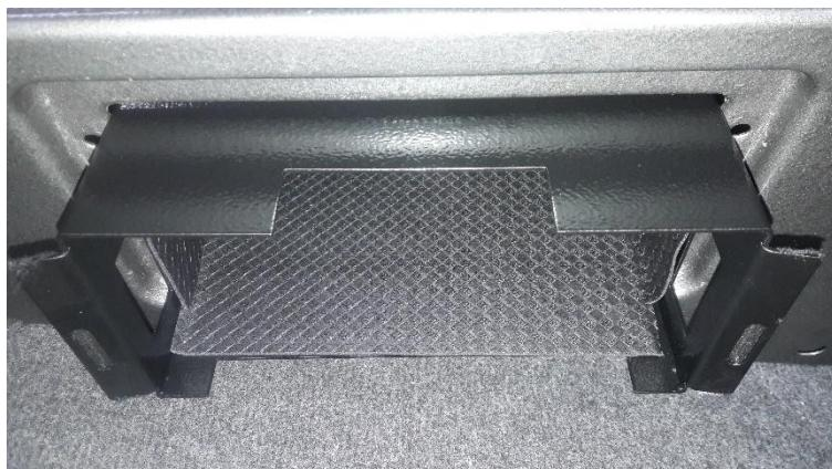
3. Then screw the box tightly to the console using the screws and nuts supplied. The holes for this are already provided in the console and do not need to be drilled separately.
