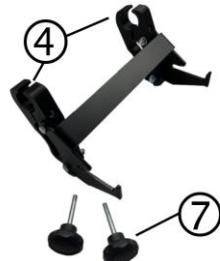
The plastic brackets (4) of the support structure must be positioned around the crossbars (5) and (6).
